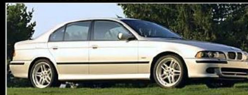
1,300 kg car is large vehicle for 50 km/h, 80 km/h & 100 km/h tests
